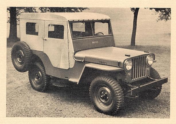
Due to the demand in the field for the ultimate in quietness and maximum year around comfort in Jeep cabs, we have developed the Super-Deluxe Jee-Cab. This deluxe Jee-Cab is insulated throughout with 3/16" beaver board, painted on both sides so that moisture will not cause distortion or discoloration. Your customers will marvel at the cab's coolness in summer, its passenger car warmth in winter and will be amazed by its quietness in operation.
