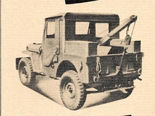
JEEP PICK-UP CONVERTED INTO A WRECKER IN 60 SECONDS
