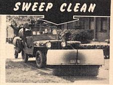
HIGH SPEED WITHOUT DUST. The Little Giant SPRINKLER holds down dust. The speed of the water pump and the flow of water corresponds to the speed of the broom — assuring proper flow whether sweeping 4 miles per hour or 8 miles per hour.
