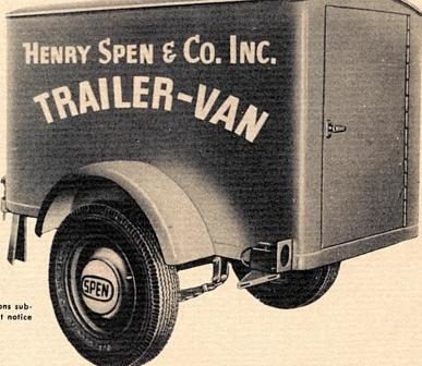
ldeal for merchants, salesmen and business people for deliveries and pick-ups. Building and maintenance men can detach trailer from vehicle and trailer can be left on the job with complete safety of tools, equipment and materials. Does the work of a truck without the expense of a truck. Body construction provides for shelves.
