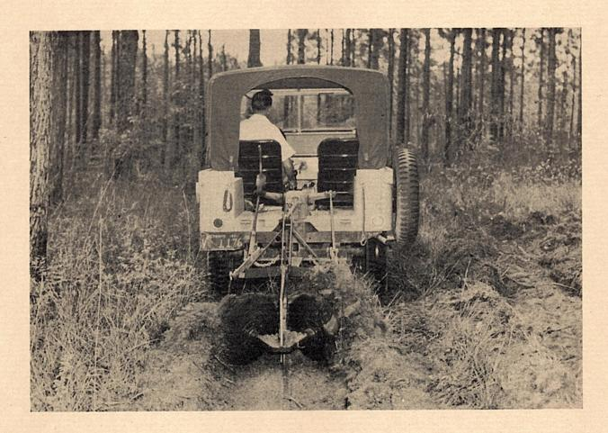
Shown above is an example of the effective work the 'Jeep' and Fire Fighter Plow do, even in thickly wooded sections. By means of the two 18" discs, a protective strip more than 5 feet wide is plowed to aid in the control of brush and forest fires.
