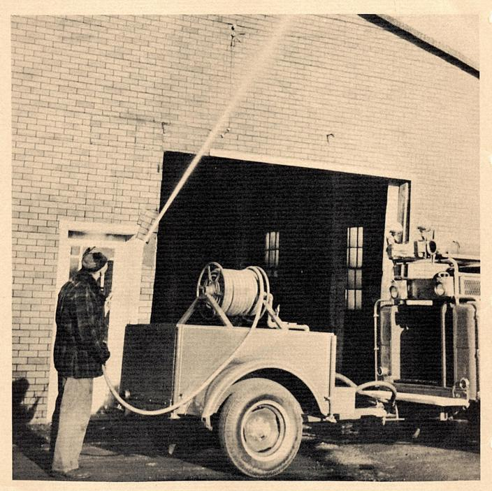
The Howe Jeep Tank Trailer, used in conjunction with the Jeep pumper, supplies a high pressure stream of water that reaches several stories high. This stream of water may be placed into immediate
