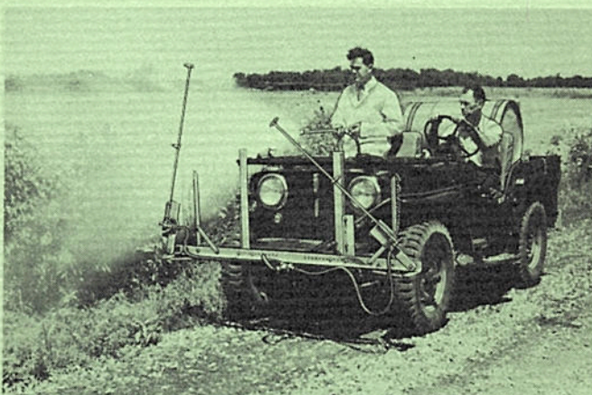
Spraying fence rows to eliminate roadside weeds, also with hand gun attachment. Note how boom ends fold up and over. Ends of booms also fold back to clear trees and posts.
