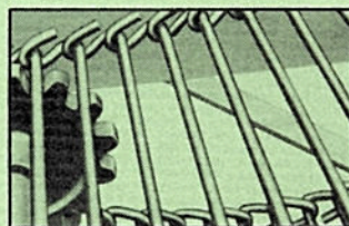
CONVEYOR CHAIN —To meet varying conditions of soil, conveyor chain can be quickly changed to level bed or elevator operation.
