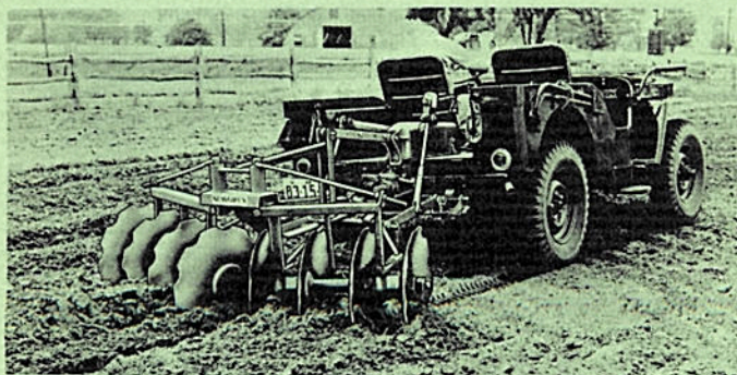
Views of the Newgren lift-type Bush and Bog Harrow in action, reworking hard, packed ground, and summer fallowing.
