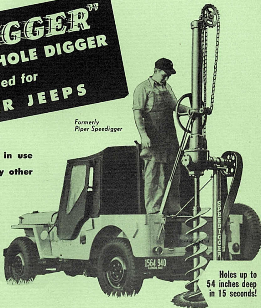
"SPEEDIGGER" in transport position, showing tilting range.
