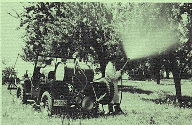
Insect control on pear trees, using hand gun attachment—half turn of handle adjusts from long stream to fine mist.
