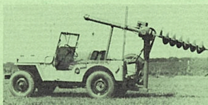
"SPEEDIGGER" in transport position, showing tilting range.
